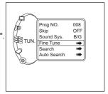
4. Press the VOL+ button to enter the Fine Tune Menu, and then the VOL- button to search downwards or the VOL+ button to search upwards until it has searched the TV signal you need.
